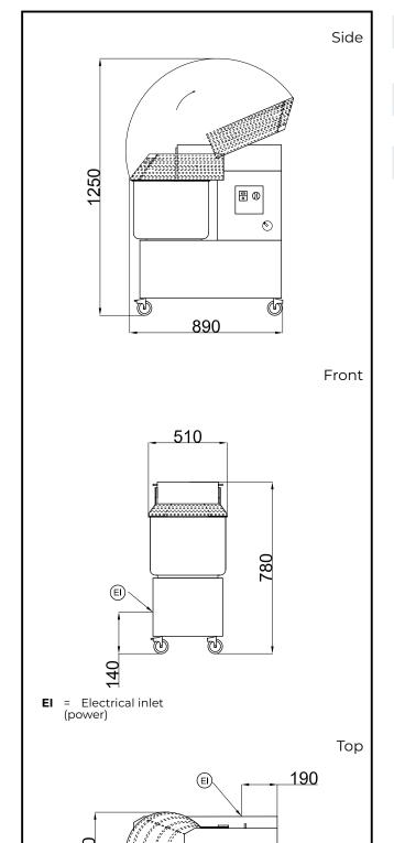
Electric Supply voltage: 380-415V/3 ph/50 Hz **Total Watts:** 2.2 kW Capacity: Maximum kneading (60% hydratation): 33 kg/Cycle Key Information: External dimensions, Width: 510 mm External dimensions, 840 mm Depth: External dimensions, Height: 780 mm 109 kg **Shipping weight:**
